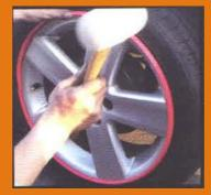
4. step Lightly tap with mallett (Insure protector is secure and flush all round lightly tap with mallett)
